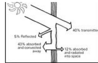
**Spectrally selective glazing** is commonly used for cooling climates or for westerly elevations where solar control and natural lighting are a priority. Spectrally selective glazing maximises light transmission while simultaneously reflecting unwanted solar radiation (UV and near infrared). Spectrally selective coatings can also have low emissivity.
