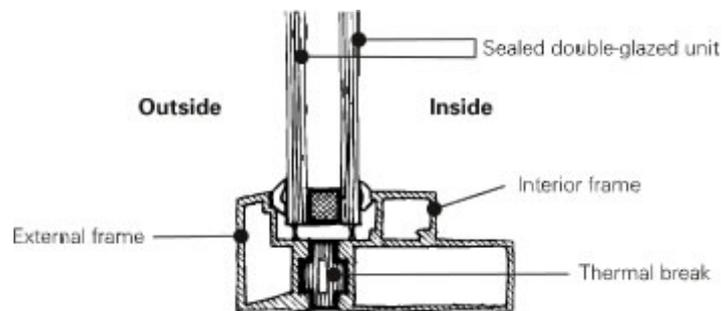
**Some manufacturers** may be able to provide aluminium frames made from recycled material, which greatly reduces the energy used during manufacture.
