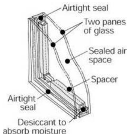
The best thermal performance for air-filled units occurs when the space between the panes is about 12 mm. If the double glazing is also to be used for noise reduction, a wider gap may be appropriate with some trade-off in thermal performance.
